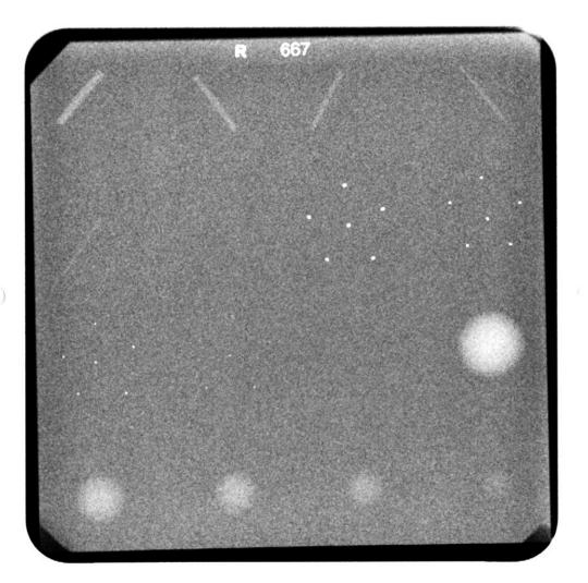
**•** Fibers **≻**1.56 – 0.4 mm nylon ♦ Masses > 2.0 - 0.25 mm**•** Microcalcs: **>** 0.54 − 0.16 mm **Phantom score: Pass** Fibers  $\geq 4$ Masses  $\geq$  3
